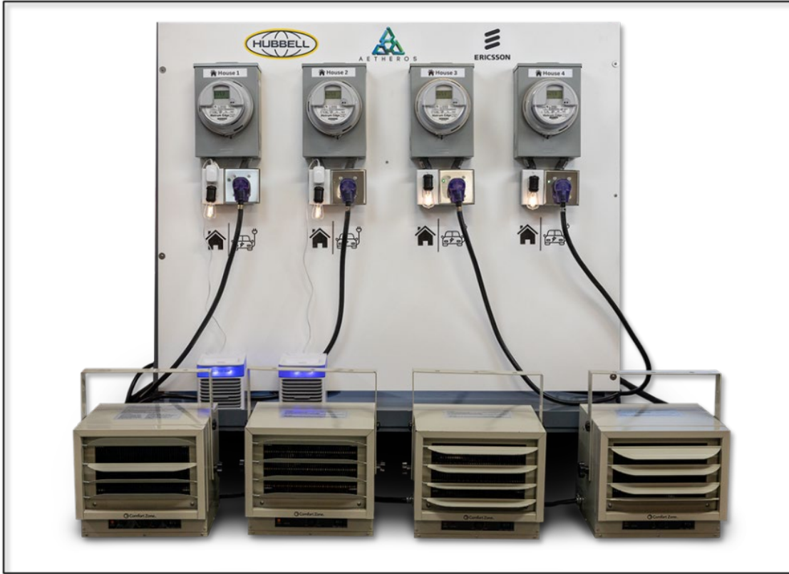
Figure 1 – Secondary Circuit Test Network
